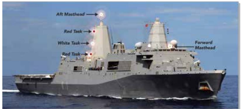
RSL technology with non-metallic luminaires used on both the LPD 17 San Antonio Class (shown above) and the Italian FREMM Bergamini Class.
